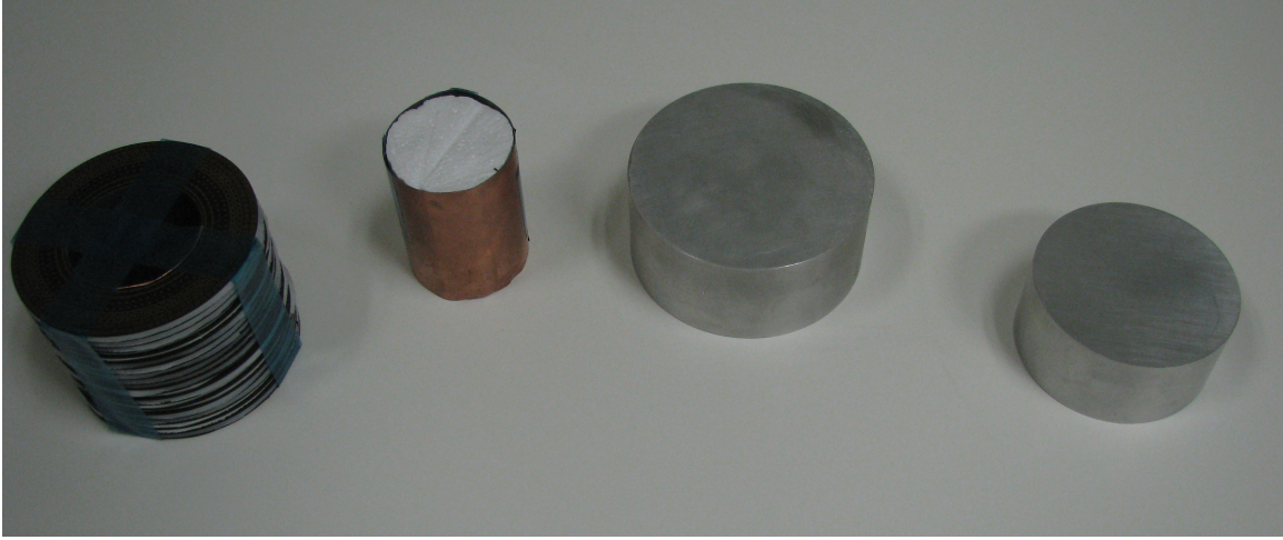
Figure 7.2: In order from left to right is the cloaked cylinder (540mm radius), bare cylinder (300mm radius), 450mm radius calibration cylinder and 375mm radius calibration cylinder.
