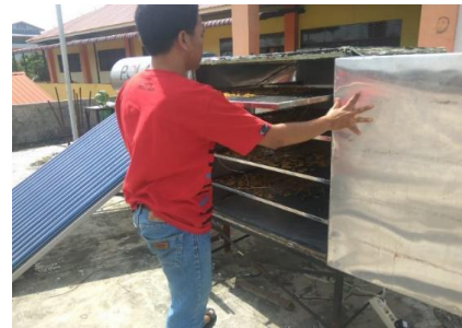
Gambar 2. Pengering Surya Tipe Kolektor Tabung Vakum ( Evacuated Tube Collector )
