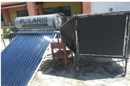
Gambar 2. Pengering Surya Tipe Kolektor Tabung Vakum ( Evacuated Tube Collector )
