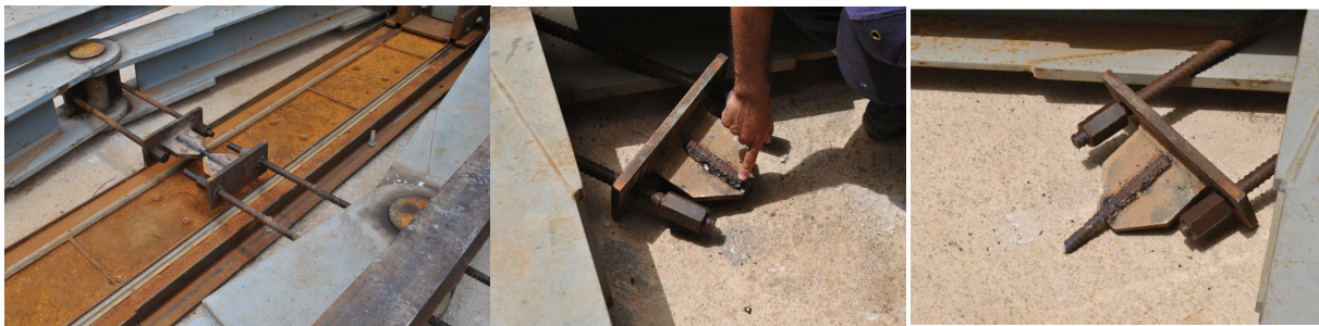
Figure 7: Fuse device before and after failure.
