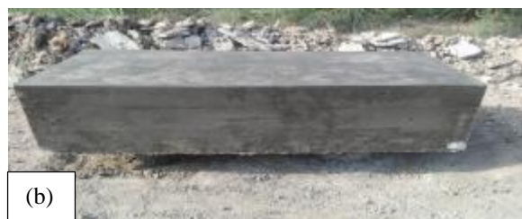
Figure 10. Schematic represented pile cap of jet grout soil-cement column group (2x2)
