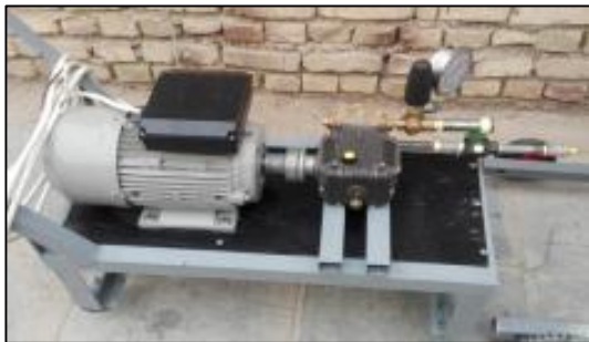
Figure 4. High pressure water jet pump
