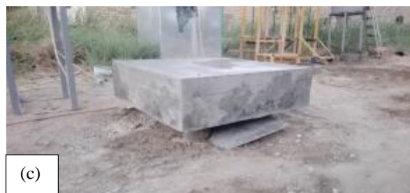
Figure 11. Cast in place pile cap of soil-cement column; (a) Single; (b) Group (1x2); (c) Group (2x2)
