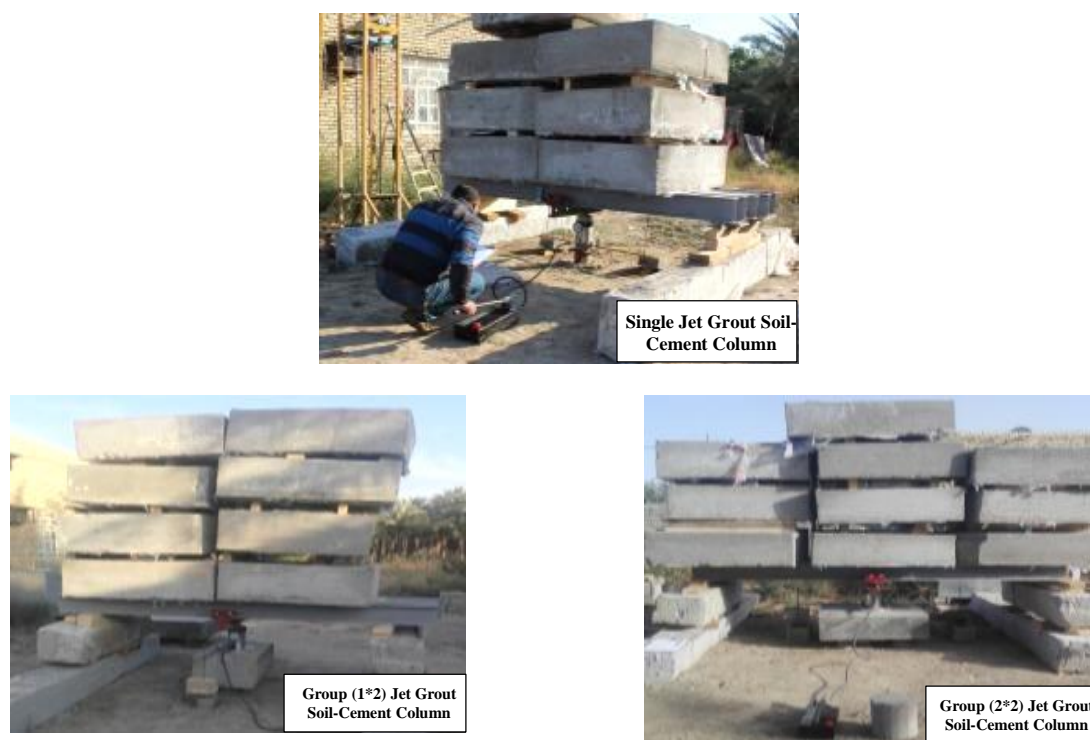
Figure 13. Pile load test for single, Group (1×2) and (2×2) jet grout soil-cement column
