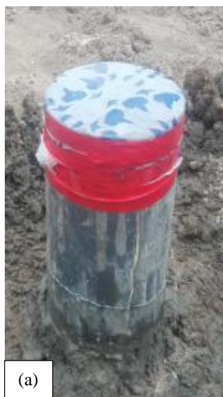
Figure 11. Cast in place pile cap of soil-cement column; (a) Single; (b) Group (1x2); (c) Group (2x2)
