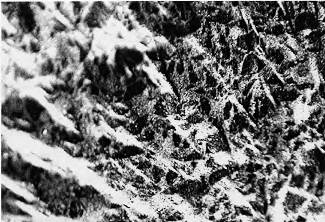
Figure 36. Photograph of the individual carbides remaining in the impact cavity.
