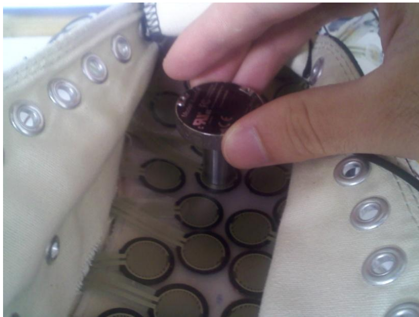
Figure 2.4 Calibrating the Sensors with a Load Cell
