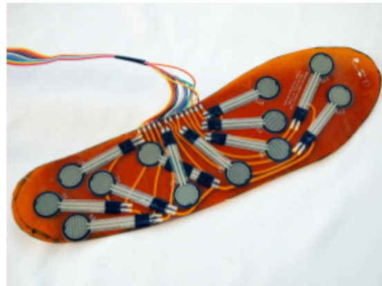
Fig. 1. The kinetic insole, including 12 force sensitive resistors mounted on flexible circuit board. Heel and toe sensors have longer copper pads to enable multiple sizes of insoles.
