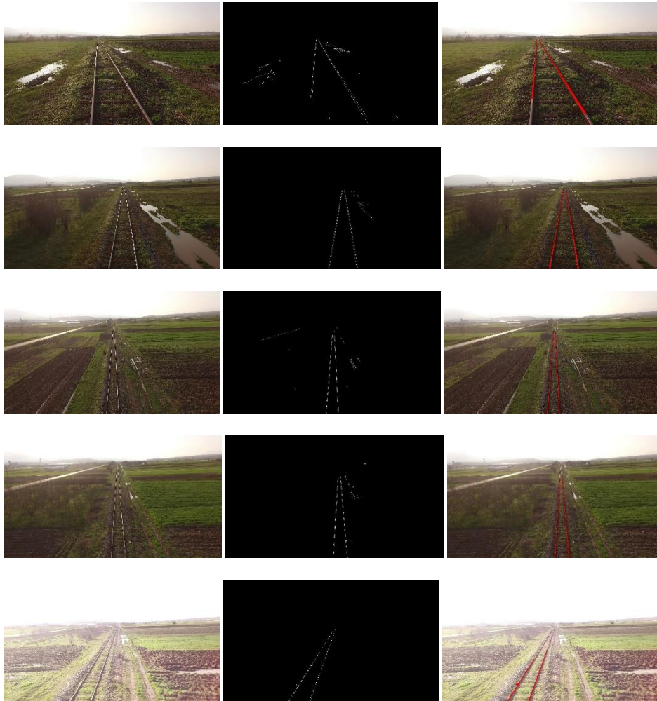
Fig. 3 Original image acquired by drone, adaptive Canny edge detection processing results and rail tracks detected
