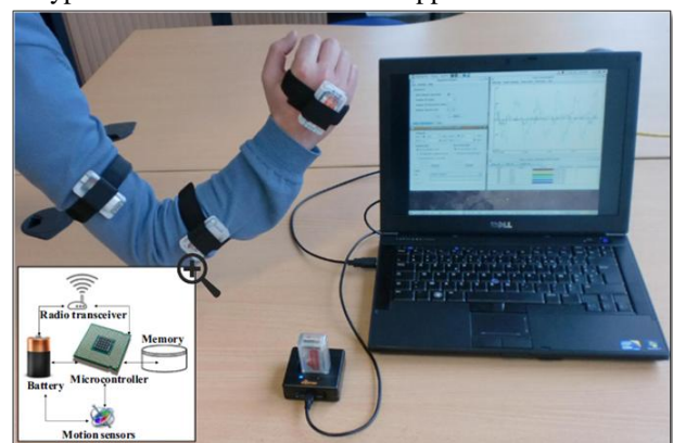
Figure 2. Prototype of WSN for Rehabilitation Application
