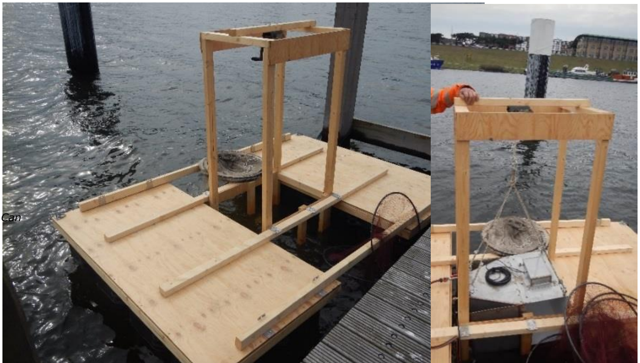
Figure 3-3 The pontoon with camera that was used at the monitoring location near the sluices of the North Sea canal near IJmuiden
