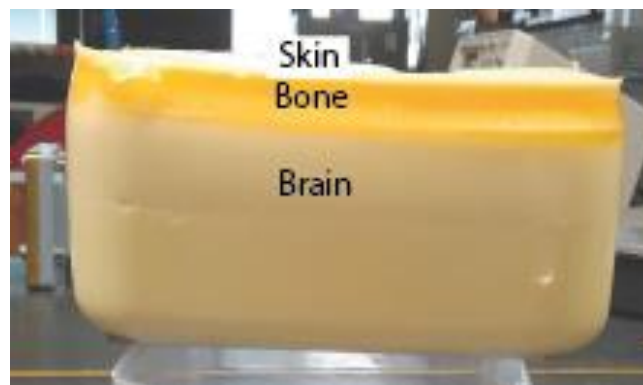
Fig. 3.2 Fabricated inhomogeneous human head phantom.
