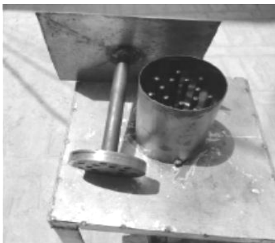
Figure 5. Top view of the compression cylinder with top circular steel plate with holes to slide inside the cylinder under the influence of sufficient load.
