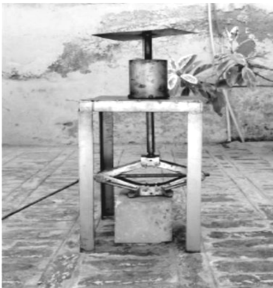
Figure 4. Coal Briquetting press machine showing the compression and jack removal mechanisms.
