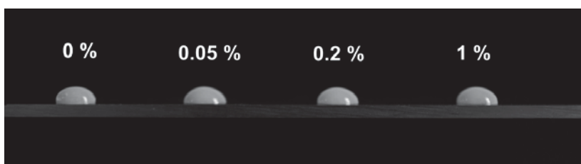
Fig. 2 – A lateral view of cured flowable nonmodified and modified samples after 10 s slumping at room temperature.
