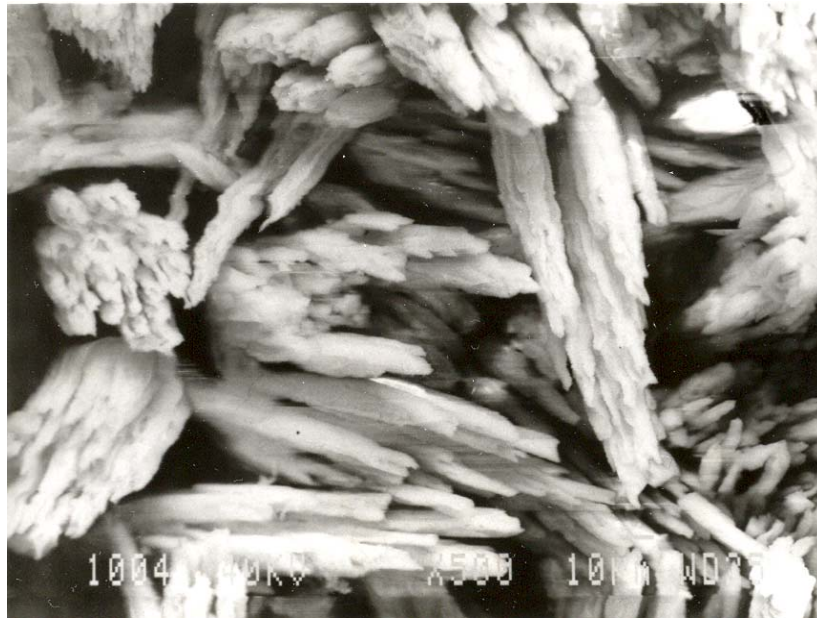
Fig. 4. SEM photograph of sample 1 of heater scale (x500)
