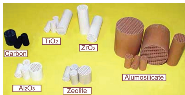
Figure 1. Monolithic honeycomb supports and catalysts [10]
