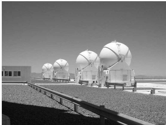
Fig. 19. Four 1.8m Auxiliary Telescopes of the VLTI (Very Large Telescope Interferometer), Paranal, Chile.
