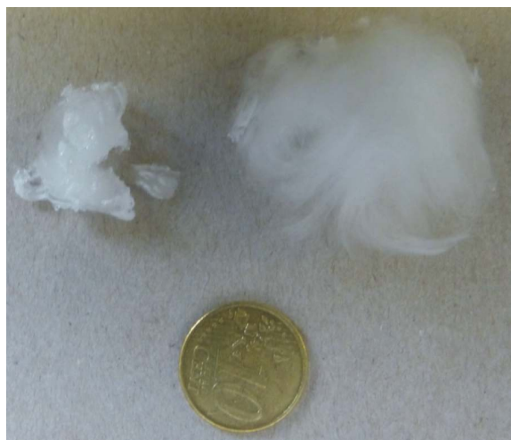
Figure 5. Comparison of plasma treated (left) and conventionally thermal treated (right) quartz wool
