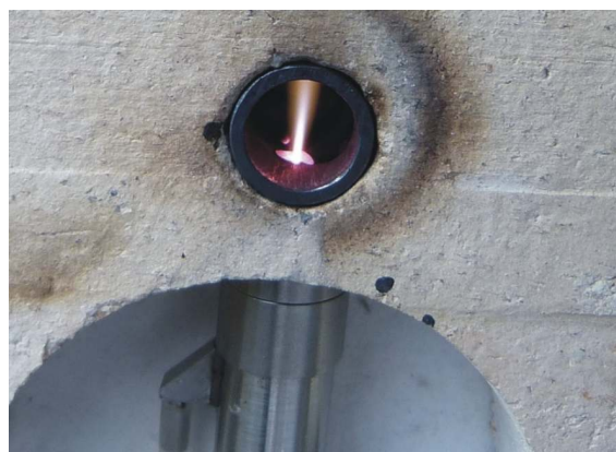
Figure 2. Plasma torch in operation inside metallic oven piece
