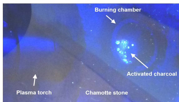
Figure 3. Plasma treatment of activated charcoal observed through a cobalt-glass
