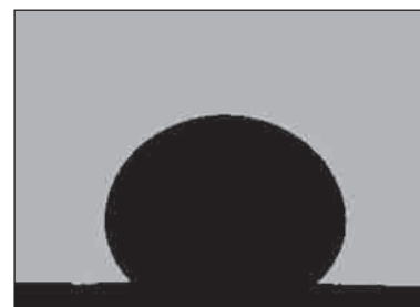
Figure 2 A Cu-40 Ag alloy drop placed on aluminium oxide surface at 1 423 K
