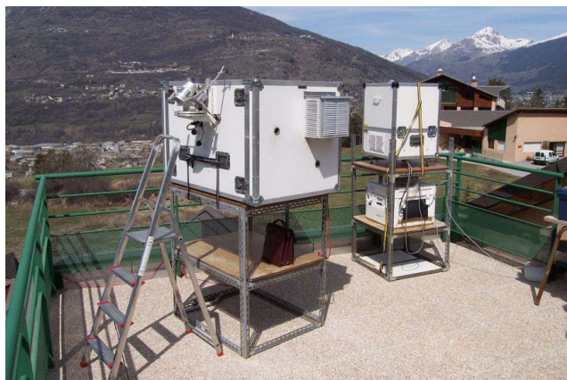
Fig. 1. The measurement platform, with the two spectroradiometers, on the left Bentham, on the right Jobin Yvon.
