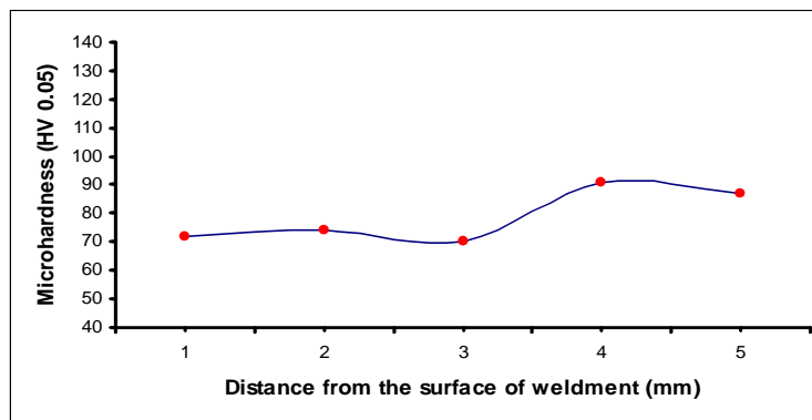
Figure (16) Microhardness distribution along plate thickness for MIG welding.
