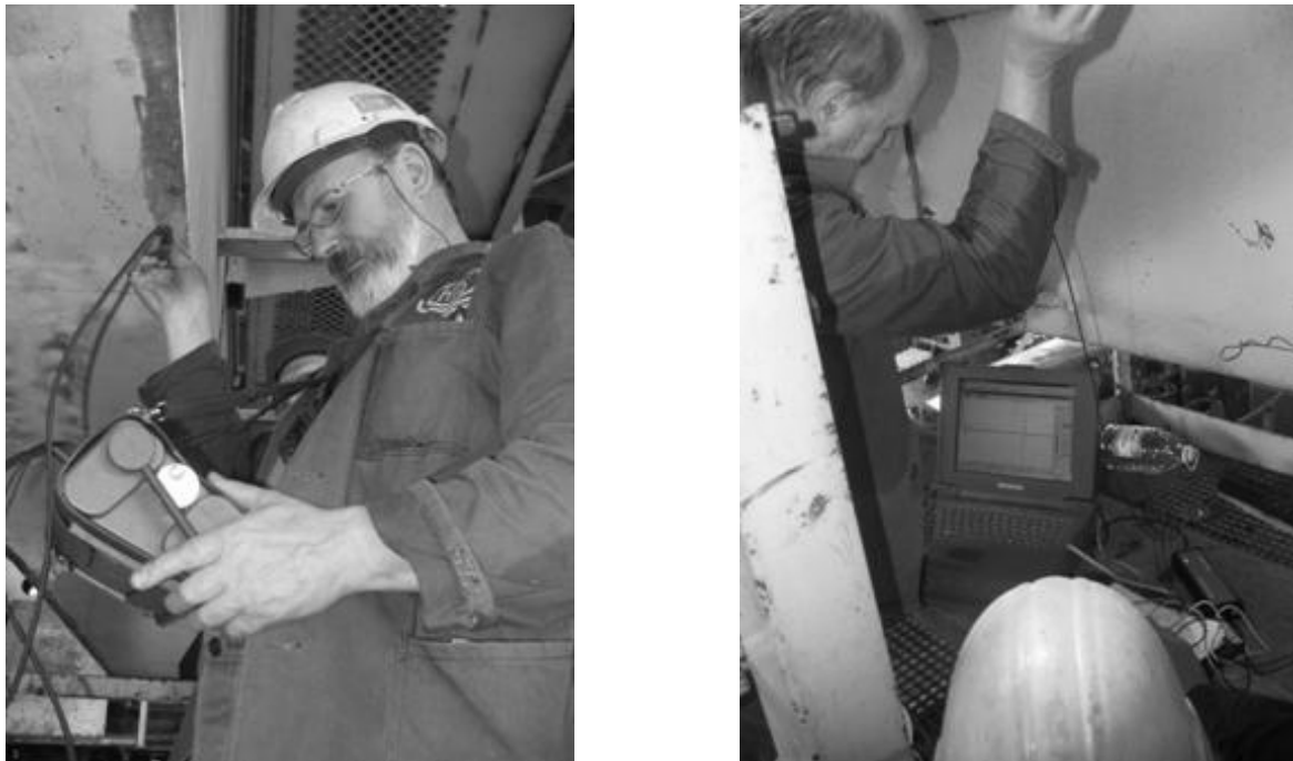
Fig. 1. Investigation with flaw detector USM-35M (left) and flaw detector USLT 2000I (right) Rys. 1. Badanie defektoskopem USM-35M (po lewej) oraz defektoskopem USLT 2000I (po prawej)
