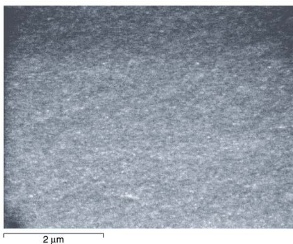
Figure 9. Surface morphology obtained by SEM of neat DGEBA
