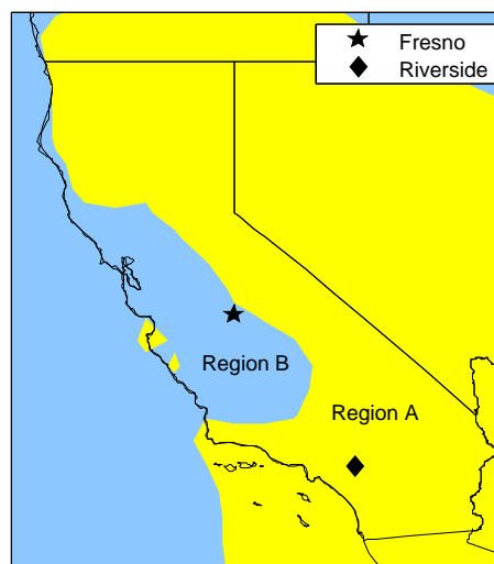
Fig. 11. California regions of high (Region A) and low (Region B) ammonia sensitivity in predicted nitrate. Region A (yellow areas in California) comprises the grid points for which predicted 2009 annual nitrate concentrations increase by 60 % or more above the base case when ammonia emissions are doubled in GEOS-Chem. Region B (blue areas in California) comprises the grid points for which predicted 2009 annual nitrate concentrations increase by less than 60 % when ammonia emissions are doubled in GEOS-Chem.
