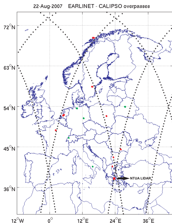
Fig. 1. NTUA's lidar station (red square) and CALIPSO ascending and descending orbits overpassing Athens (cross lines), on 22 August 2007. All the other EARLINET stations are reported as red dots for "case 1" and "case 2" and green dots for "case 3", according to CALIPSO correlative measurement strategy of EARLINET.
