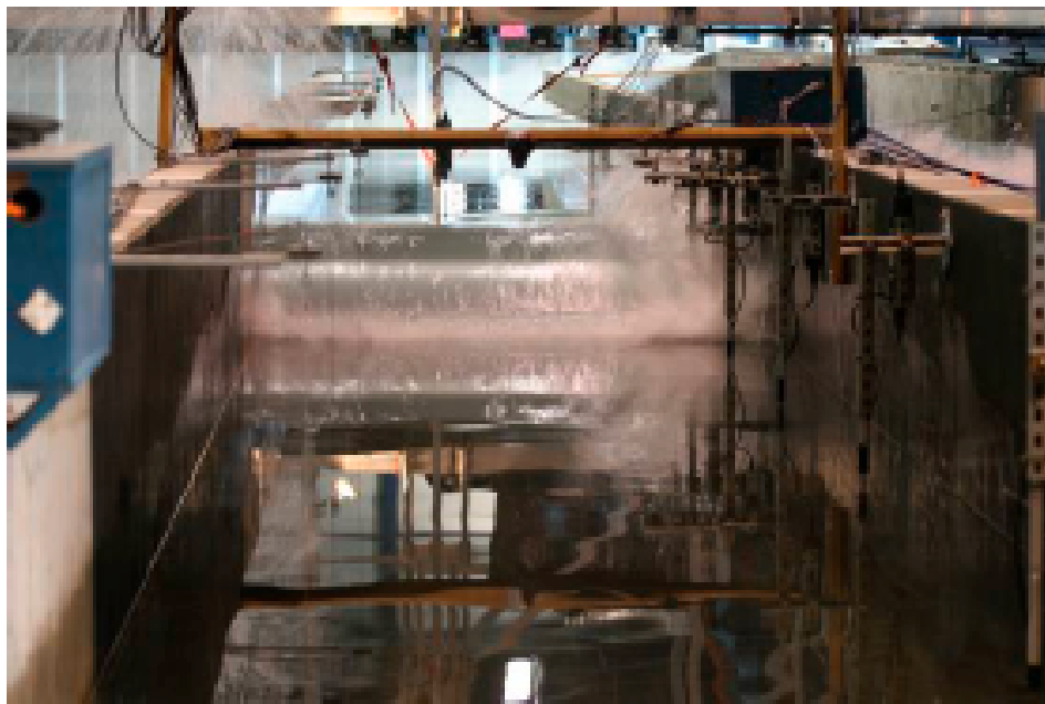
Figure 5. A solitary breaking wave in one of two flume channels instrumented to measure run-up.
