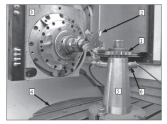
Figure 1 Investigation scheme: 1 - gear wheel, 2 - the head, 3 - the machine tool spindle, 4 - rotatable table, 5 - fixture of the gear wheel
