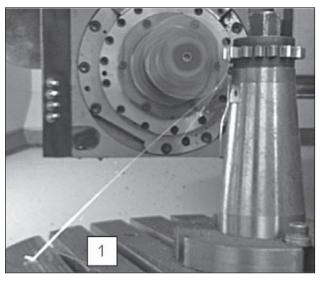
Figure 7 Backward machining of the left tooth sides
