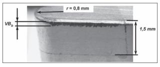
**Figure 5** A CBN insert wear image where:  $L = 64 \text{ m}, f_2 = 0,09 \text{ mm}$
