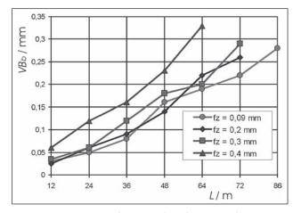
**Figure 6** Tool wear as a function of the feed value  $f_z/mm$ ; q = 0,1 mm
