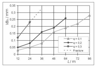
**Figure 3** Tool wear for feed  $f_{z} = 0,09$  mm
