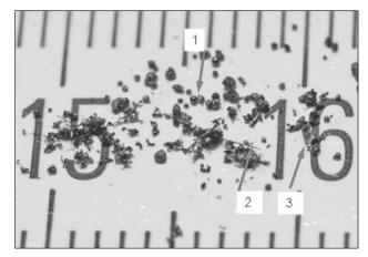
Figure 9 Geometrical forms of the chips
