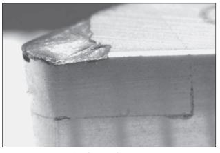
**Figure 4** Cutting wedge fracture for  $q = 0.3 \text{ mm}, f_2 = 0.09 \text{ mm}$
