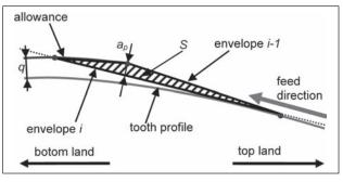
Figure 2 Geometry of the removed layer
