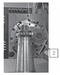
Figure 8 Forward machining of the right tooth sides
