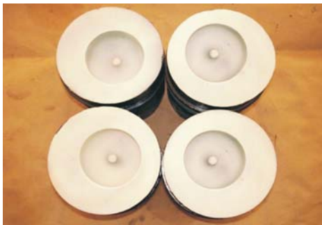
Figure 1. Photographic view of piston top with ceramic coating
