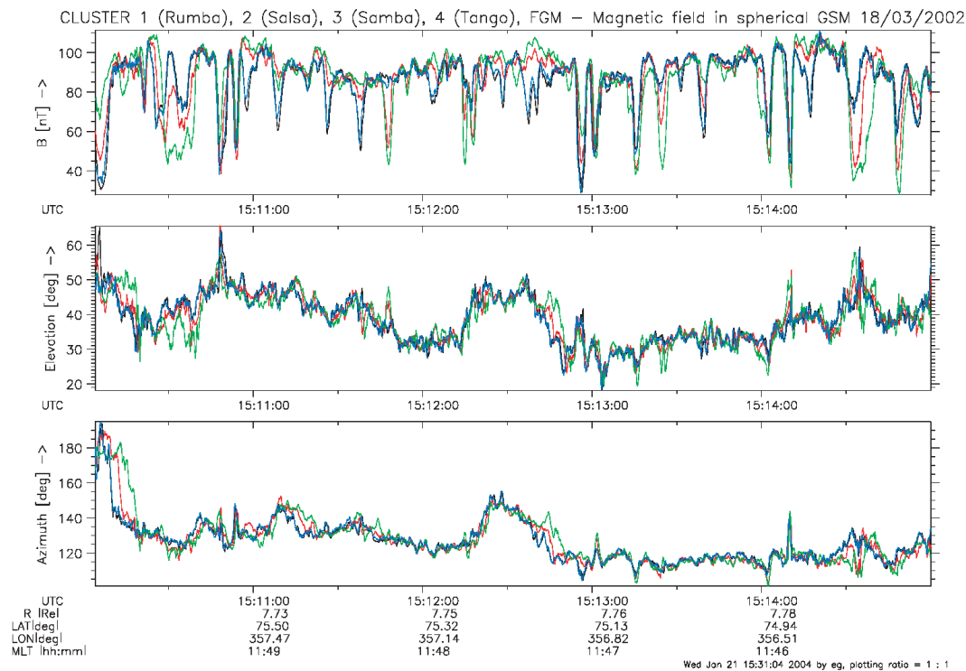
Fig. 2. A sequence of mirror mode structures similar to the AMPTE sequence as measured by the Cluster quartet in the magnetosheath (taken from Lucek et al., 2001). The deep nonlinear dropouts in the magnetic field from an in the average high magnetic field value are seen. Also seen is the weak variation of the magnetic field over the small separation distances of the Cluster spacecraft fleet. The variation is mainly in one component only as can be realized from the much more gradual (background) variations in elevation and azimuth of the magnetic fields.
