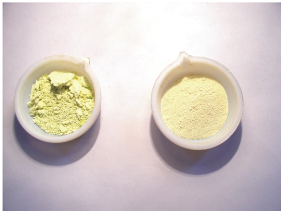
Figure 2. The photograph of UO_2F_2 after a long contact with water vapors (left) and after the removal of water (right)
