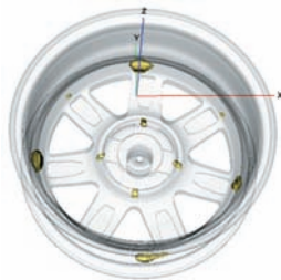
Fig. 13 Predicted shrinkage defects under forced-cooling
