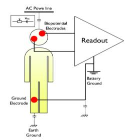
**Figure 6.** A biopotential readout circuit linked to the biopotential electrodes to extract the electroencephalogram signals.
