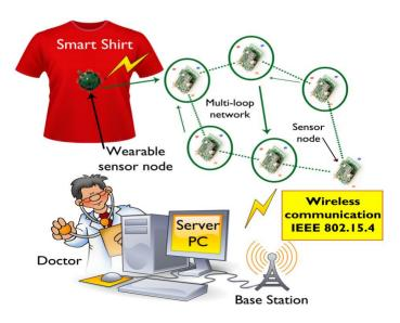
Figure 5. The system architecture with a wearable smart shirt.
