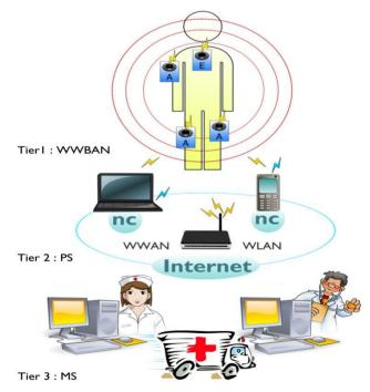
The second stage includes the personal server application that runs on a personal digital assistant, cell phone or home personal computer. The personal server is responsible for a number of targets, providing an interface for wireless medical sensors, users and the medical server. The interface to the WWBAN includes network configuration and management features. The network configuration includes the objectives: a sensor node registration (type and number of sensors), initialization (e.g., to
