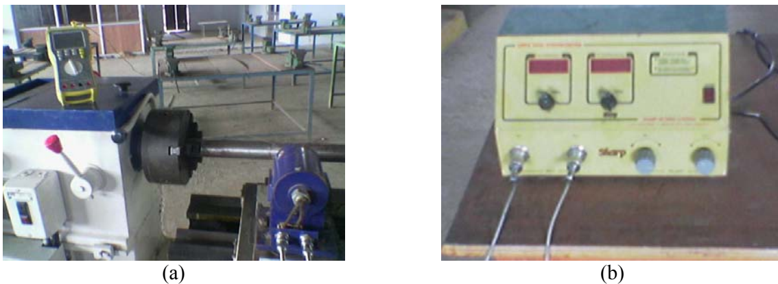
Fig. 1. Experimental setup (a) Turning tool dynamometer (b) Display channel for turning forces
