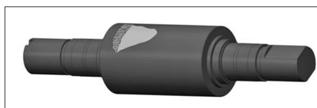
Figure 1 A Cat's Tongue Spall visible on working roll surface layer
