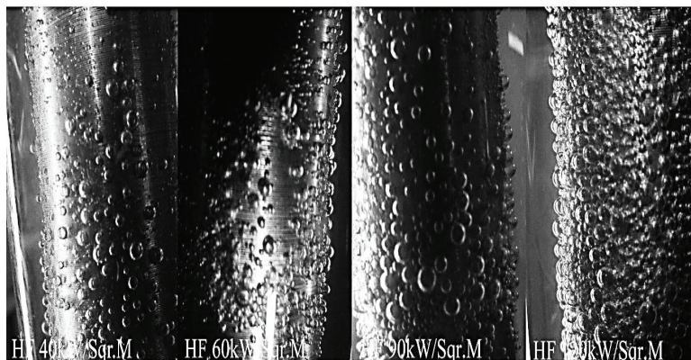
Figure 6. Bubble generation at various heat fluxes for ethanol/water solution.
