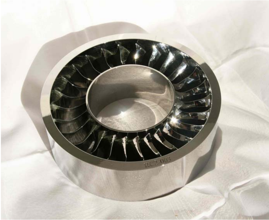
Fig. 5 – Straightener for a helicopter gas-turbine engine. PEP / Turbomeca / Best in Class
