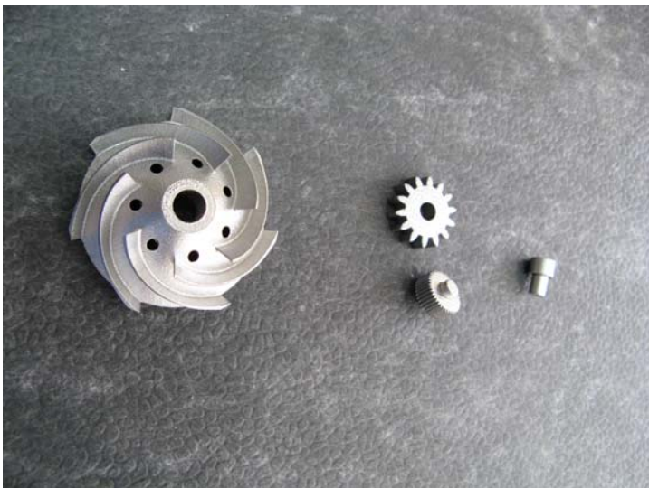
Fig. 6 – Examples of parts built in EOS superalloy CoCr MP1 on INCDMTM for industry
