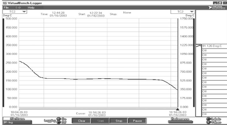
Figure 3 Cooling curve, sample AISi12Cu, 40 Kg, cooling time 54 min. (soft LabView)
