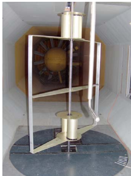
Fig.3 – Combined Darrieus-Savonius rotor tested in the subsonic wind tunnel
