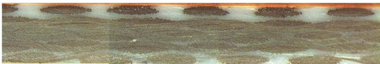
Figure 3. Light microscopic image of a srPET sample's cross section showing a good impregnation ( T_c 225°C/ t_h 6.5 min)
