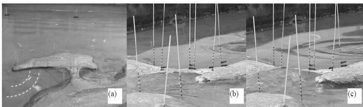
Fig. 12 (a) Edge wave propagation along the coastline, (b) and (c) show the flooding and overflow at the north side of the tombolo while the edge wave propagation from the south side was still going on.
