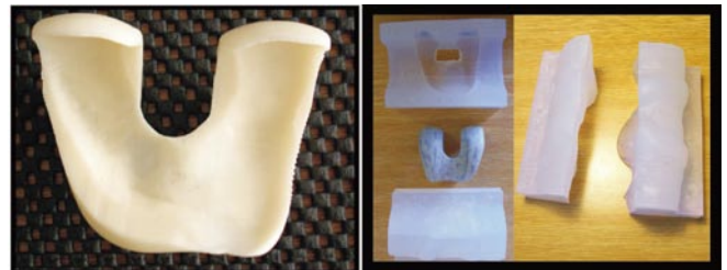
Fig. 7: Printed ABS model of knee joint replacement (left) and silicon mould (right)
