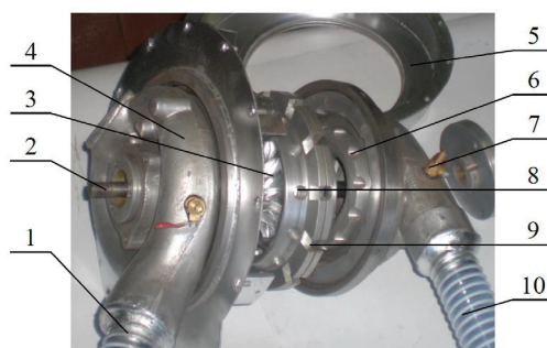
Fig. 4. Structure of the homogenizing unit of the pulsation machine with a vibrating rotor: 1 – branch pipe of the product discharge; 2 – rotor axis; 3 – vanes; 4 – body; 5 – cover; 6 – stator; 7 – pass valve; 8 – openings of the rotor; 9 – grooves of the rotor; 10 – branch pipe of the product supply
