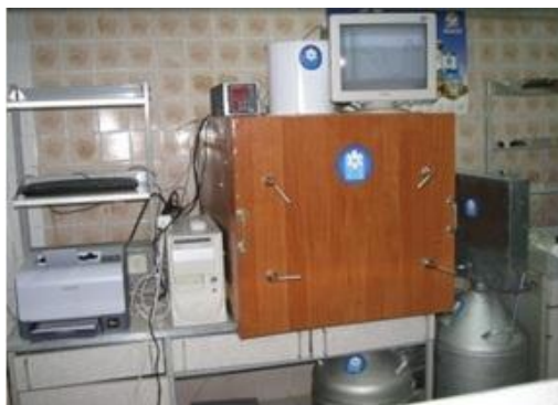
Fig. 1. Cryogenic programmed freezer with software
