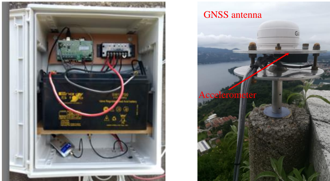
Figure 9. Design and implementation of a multi-sensor control unit in a monitoring site.
