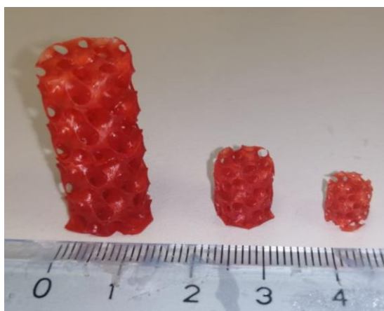
Figure 4. Gyroid-like structures printed with P_Bmim[BF 4 ].
