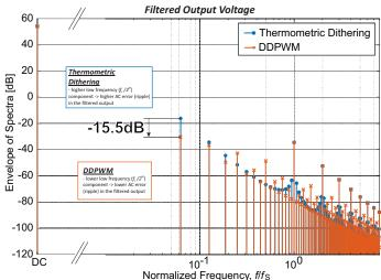
Fig. 7. Envelope of the spectra of N=4-bit DPWM with M=5 bit thermometric dithering over  $2^M$  periods as in Fig.2 and of N+M DDWPM patterns, filtered by a  $2^{\rm nd}$  order LC filter, as in the buck converter in Fig. 1, with corner frequency  $2\cdot 10^{-2}f_{\rm s}$ .
