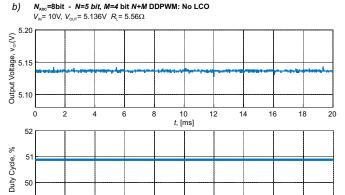
Fig. 11. Output voltage waveforms and duty cycle waveforms of the synchronous buck at  $f_{\rm s}=100{\rm kHz}$  switching frequency and  $f_{\rm clk}=3.2{\rm MHz}$  digital clock frequency for  $N_{\rm ADC}=8$ : a) using plain DPWM at N=5 bit resolution and resulting in LCOs, b) using N+M bit DDPWM with N=5 and M=4, revealing LCO suppression.
