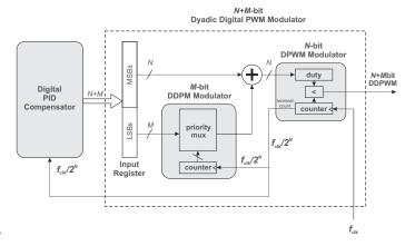
Fig. 5. Architecture of the proposed DDPWM modulator.
