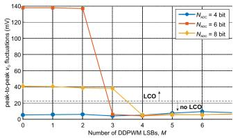
Fig. 12. Amplitude of LCOs for N+M-DDPWM with N=5 under different values of M for  $N_{\rm ADC}=4$ ,  $N_{\rm ADC}=6$  and  $N_{\rm ADC}=8$ , open-circuit load.
