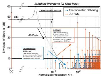
Fig. 6. Envelope of the spectra of N=4-bit DPWM with M=5 bit thermometric dithering over  $2^M$  periods as in Fig.2 and of N+M DDWPM patterns.
