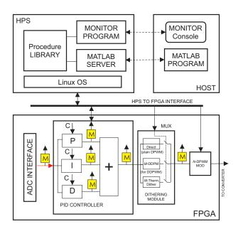
Fig. 10. Internal Hardware/Software organization of the SOC system.
