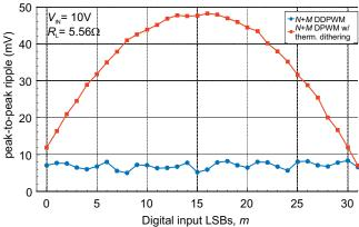
Fig. 15. Measured dithering-induced ripple voltage (open loop configuration) vs. hi-res duty cycle by the thermometric dithering (Fig.2) and by DDPWM (Fig.4) under the same M=5 resolution enhancement.
