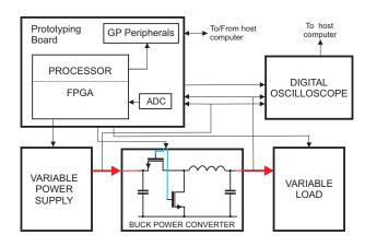
Fig. 9. Block diagram of the experimental testbench.
