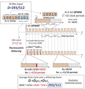
Fig. 2. High resolution DPMW by thermometric duty cycle dithering over  $2^{\hat{M}}$  switching periods.
