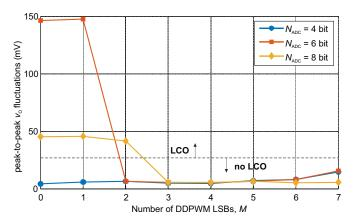
Fig. 13. Amplitude of LCOs for N+M-DDPWM with N=5 under different values of M for  $N_{\rm ADC}=4$ ,  $N_{\rm ADC}=6$  and  $N_{\rm ADC}=8$ ,  $I_{\rm O}=1{\rm A}$  load current.
