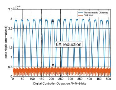
Fig. 8. Simulated dithering-induced ripple voltage in open loop configuration (normalized with respect to the DC output voltage) vs. hi-res duty cycle by M=5 bit thermometric dithering (Fig.2) and by N=4-bit, M=5 bit DDPWM (Fig.4).
