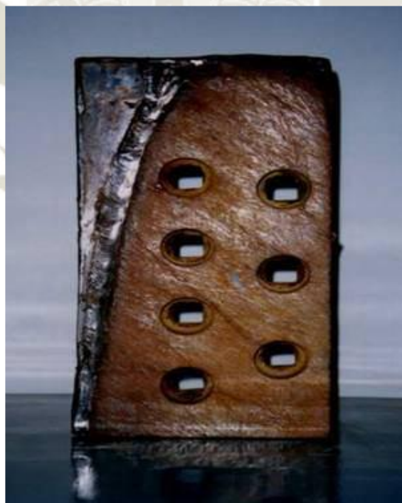
Figura 2-35 - Recalce de cantonera de tractor Cat - D8T [6]
