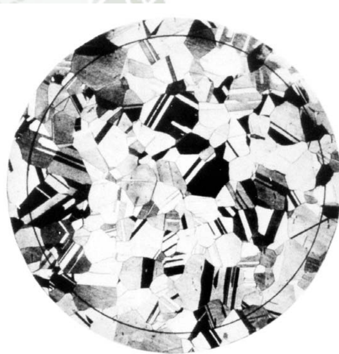
FIG. 3 Example of Twin Grains (Contrast Etch) from Plate III. Grain Size 0.090 mm at 75X
