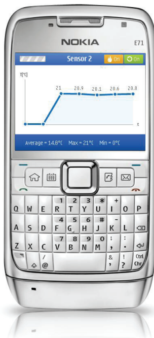
Fig. 5 Remote temperature monitoring
