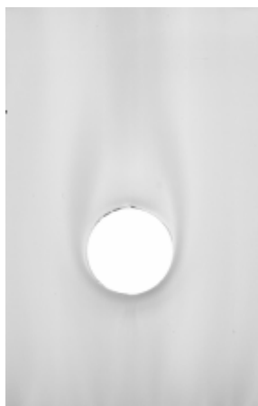
Figure 2. Boundary layer visualization for flow around single sphere ( Re_{p,0} = 2800 ).
