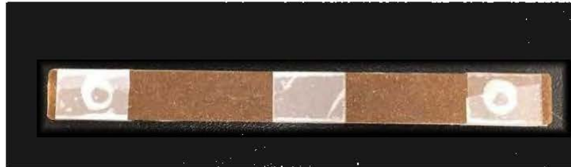
Figure 2.6 Le mode de fixation de composite sandwich CBP-Al-CBP.
