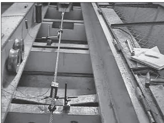
**Figure 4** Acoustic method measurement set up. Display of the measurement part of the set up – microphones and deviation gauger.
