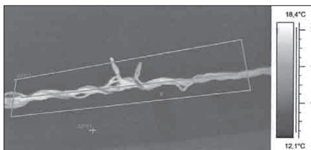
**Figure 6** Ruptured steel wire rope. Thermogram – transformed infrared field into visible spectra.
