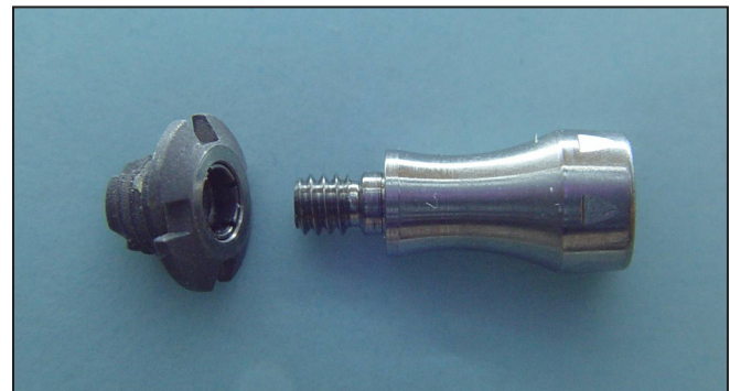
Figure 1. A typical 2.5 mm long craniofacial implant (Straumann USA, Inc., Andover, MA, USA), with its percutaneous titanium abutment, and integrated by welding, attached stainless steel keeper on right side (Technovent Ltd., Leeds, England).
